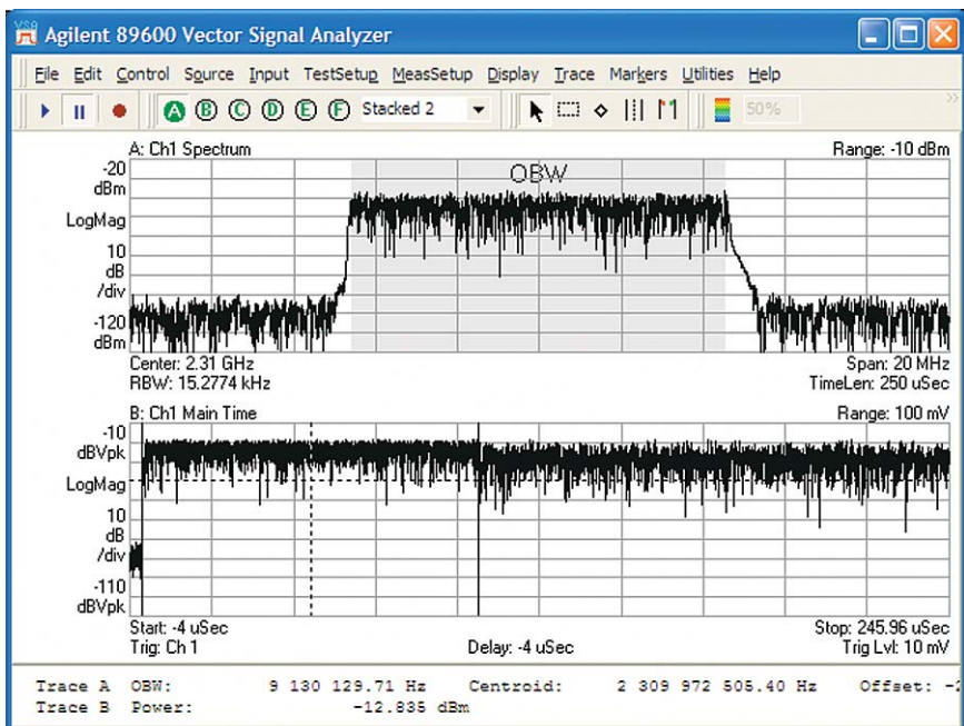
Figure 2. Occupied bandwidth and band power measurements; numeric results are shown at the bottom of the display.
